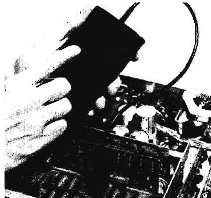
10529A Logic Comparator—an in-circuit IC functional tester.
