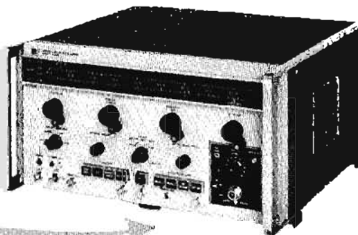
The 8690B Sweep Oscillator offers exceptional value in performance, operation and versatility. The 8690B mainframe provides complete flexibility with start/stop, ΔF, and marker sweep along with CW operation and AM and FM capability. The complete family of solid state and BWO plug-ins shown below, accent this value with coverage from 400 kHz to 40 GHz. Dimensions: 8¾" (222 mm) high, 18¾" (467 mm) deep, 16¾" (425 mm) wide. Weight: net, 49 lbs (22,2 kg); shipping, 59 lbs (26,8 kg). Price: $1700.
